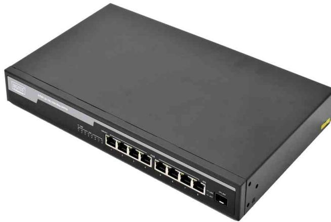
Gigabit Ethernet PoE Switch, 8-Port, 1x SFP Uplink
